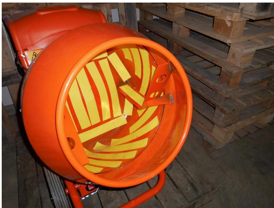
Figure 2. Cement mixer used for assessing skinset
